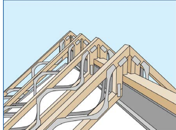
RD05: Solid Trimmers installed perpendicular to roof slope allows face fix hangers to trim openings
